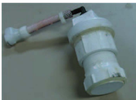
Fig. 2 The porous ceramic disk was mounted in a PVC housing to facilitate the gas flow through the ceramic disk
